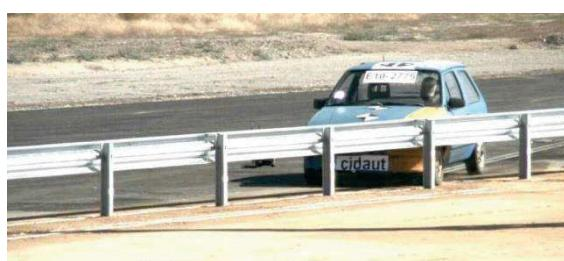
**Test:** TB11 (car 900 Kg., 100 Km/h, 20°)
