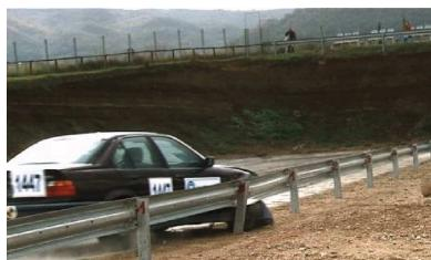
**Test:** TB32 (car 1.500 Kg., 110 Km/h., 20°)
