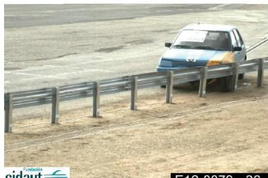
**Test:** TB11 (car 900 Kg., 100 Km/h., 20°)
